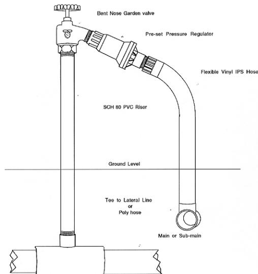
**Hypothetical Example:** A particular lateral line has 20 sprinklers. Testing has shown that the given sprinklers have an average flow rate of 25 gph. The combined output for the above line would be 500 gph (25 gph X 20 sprinklers = 500 gph), OR 8.3 gallons per minute (500 gph / 60 minutes = 8.3 gpm). Thus the proper pressure regulator for this application should have an output of at least 8.3 gpm at 20 psi.
