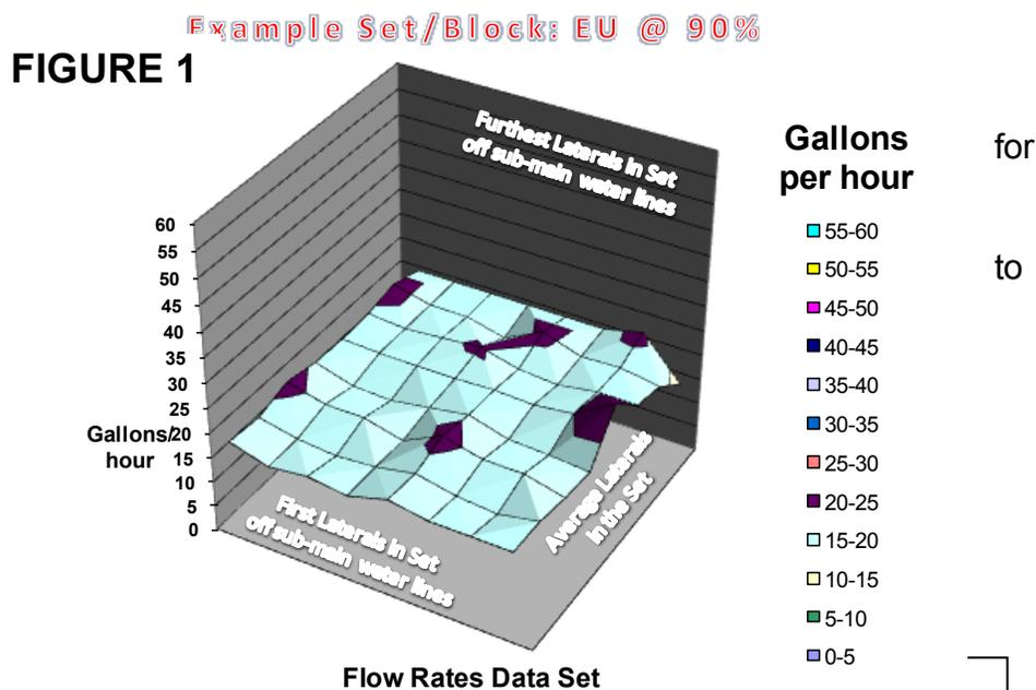
corresponding height of each intersecting line relative to the graph's y-axis indicates the amount of water (in gallons per hour) each sprinkler emitted during the time when the data was collected.
